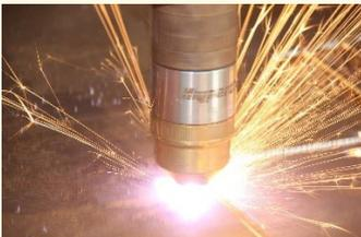
The machine created for cutting with high definition plasma source such as HPR-130XD or Hi-Focus-130(160)i.
