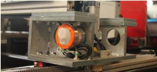
Automatic lubrication system of all moving axis
