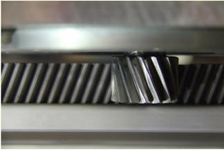
The moving system with helical style High-Precision Rack & Pinion ATLANTA (USA-DE) drive Systems. Precision Planetary reducer Neugart (DE)
